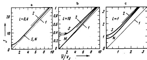
FIG. 1. CVC of filaments for different values of their lengths. The symbols S and N denote the cases  $T < T_c$  and  $T > T_c$ , respectively. The parameter  $A$  is equal to unity, which corresponds to  $T_c = T_{cB}$  for S-filaments and  $T = (T_c + T_{cB})/2$  for N-filaments. The straight line 1 corresponds to  $\bar{V} = IR_N$ , and the straight line 2 corresponds to  $\bar{V} = IR_N - 2\epsilon V_J$ .
