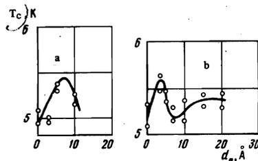
FIG. 6. Critical temperature of technetium films ( $d = 50 \text{ \AA}$ ) as a function of the thickness of the sublayer of artificial diamond for samples with different thickness of the diamond covering: a)  $d_C = 40 \text{ \AA}$ , b)  $d_C = 10 \text{ \AA}$ .
