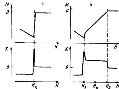
FIG. 5. Magnetization and magnetic susceptibility during the transition from the superconducting to the normal phase in a magnetic field: a) type-I superconductor ( $\sigma > 0$ ); b) type-II superconductor ( $\sigma < 0$ ).
