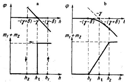
FIG. 3. Dependence of thermodynamic potential and total magnetization on magnetic field intensity near the transition from the antiferromagnetic to the paramagnetic state: 1) first-order transition ( $\delta > 0$ ); b) second-order transition ( $\delta < 0$ ).
