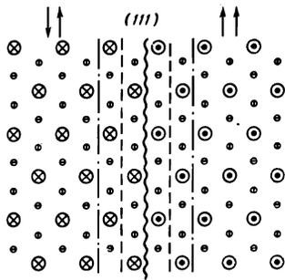
FIG. 7. Model of the interface between antiferromagnetic (left) and paramagnetic (right) phases. The large circles represent reversed ( $\odot$ ) and unreversed ( $\otimes$ ) spins of a single (111) layer; the small circles represent magnetic ions of the two neighboring layers.
