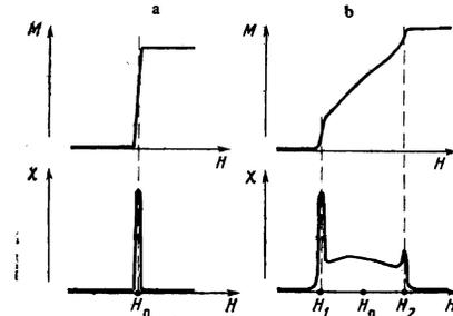
FIG. 6. Magnetization and magnetic susceptibility during the transition from the antiferromagnetic to the paramagnetic phase in a magnetic field: a) first-order transition ( $\sigma > 0$ ); b) second-order transition,  $\text{FeCO}_3$  ( $\sigma < 0$ ).
