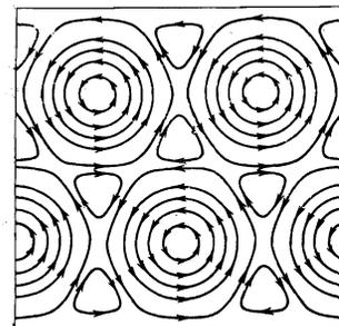
FIG. 4. Distribution of the effective exchange field produced by ions with reversed spins in the (111) plane.
