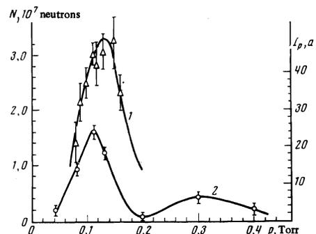
FIG. 2. Yield of neutrons in the reaction  $C_6^{12}(d, n)N_7^{13}$  (curve 1) and value of proton current (curve 2) as a function of gas pressure in the drift chamber.
