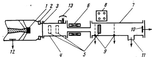
FIG. 1. Basic experimental arrangement: 1—plane graphite cathode, 2—shunt for current measurements, 3—titanium anode foil (50  $\mu$ ), 4—acceleration section of drift chamber, 5—graphite target, 6—magnet for deflection of electrons, 7—measuring section of drift chamber, 8—paraffin block with counters for neutron detection, 9—collector grids, 10—Faraday cup, 11—pumping system, 12—capacitance probe for measurement of voltage on diode gap, 13—system for admission of gas and pressure measurement.
