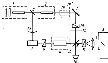
FIG. 2. Experimental setup: 1—ruby laser used as light source, 2—ruby laser used as light amplifier, 3—dye laser, 4—cell containing potassium vapor, 5—spectrograph, 6—8—mirrors, 9—11—polarizers, 12—quarter-wave plate, 13—cylindrical lens, 14—cell containing nitrobenzol, 14'—FS-6 filter, 15—diaphragm, 16—type IKT-1M energy meter.
