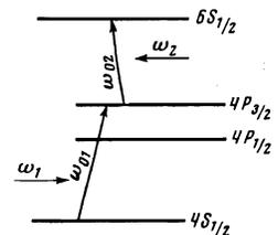
FIG. 1. Relevant portion of the potassium level scheme.
