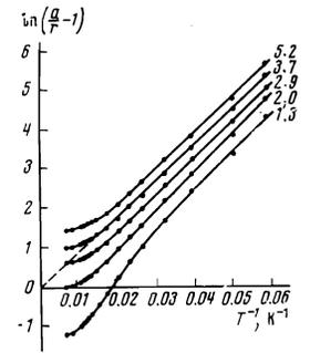
FIG. 5. Process of fitting Eq. (5) to the experimental points of curve 1, Fig. 1 (copper single crystal). The corresponding values of  $a/r_{\max}$  are given at the curves.
