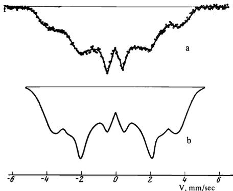
FIG. 3. Experimental (a) and model (b) Mössbauer spectra at 300°K. The method of constructing the model spectrum is explained in the text. The solid line (a) represents freehand averaging of the points. Zero velocity is taken to be the position of the center of gravity of the spectrum of pure Fe at 300°K.
