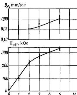
FIG. 4. Position of the center of gravity  $\delta$  of the Mössbauer spectrum and the effective hyperfine field ( $H_{\text{eff}}$ ) for the Fe atoms as a function of the number  $N$  of the Ni atoms in the nearest surrounding.
