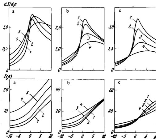
Dependence of  $I(\beta)$  and  $dI/d\beta$  on  $\beta$ : a)  $a_0(\mathbf{p}_c) = -1/2$ ; b)  $a_0(\mathbf{p}_c) = 0$ ; c)  $a_0(\mathbf{p}_c) = 1$ . Curves 1— $\gamma = 0$ ; curves 2— $\gamma = 1$ , curves 3— $\gamma = 2$ , curves 4— $\gamma = 5$ .
