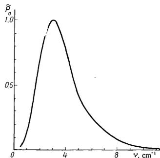
FIG. 2. The dependence of the DFR power  $P_0$  on the radiation frequency  $\nu = 1/\lambda$  for a fixed transverse dimension  $a$  of the induced-polarization region. For a Gaussian transverse distribution of the polarization the maximum value is attained at the wave number  $k = \sqrt{3}/a \sin \theta_0$ .
