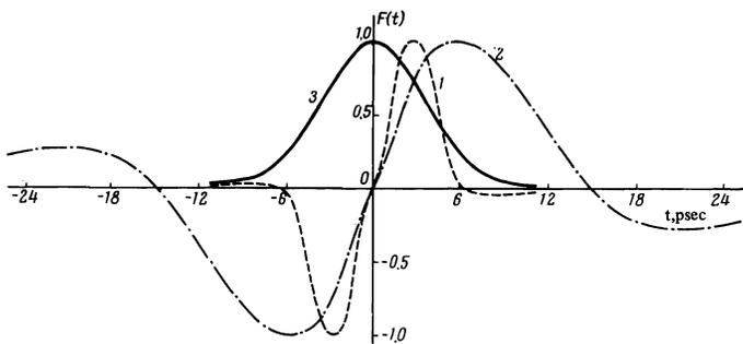
FIG. 3. The shape of the DFR pulses emitted at the Cerenkov angle for different widths a: 1)  $\tau_0 = a^{-1} \sin \theta_0 = 1.6$  psec and 2)  $\tau_0 = 16$  psec. The curve 3 corresponds to an exciting beam with the Gaussian shape of a pulse of width  $\tau_1 = 5$  psec.
