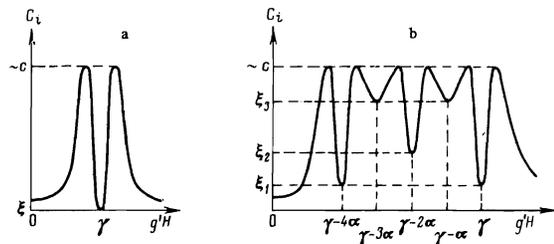
FIG. 4. Dependence of  $C_i$  on  $H$ : a)  $S' = 1/2, T \ll \gamma$ ; b)  $S' = 3/2, T \ll \alpha$ . Notation:  $\xi = c(\beta\gamma)^2 e^{-\beta\gamma}$ ,  $\xi_1 = 2c(\beta\gamma)^2 e^{-2\beta\alpha}$ ,  $\xi_2 = 4c(\beta\alpha)^2 e^{-2\beta\alpha}$ ,  $\xi_3 = 2c(\beta\alpha)^2 e^{-\beta\alpha}$ .
