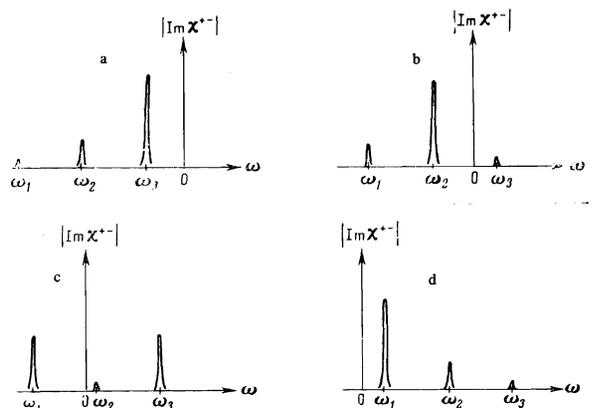
FIG. 5. Change of the ferromagnetic resonance lineshape with variation of the magnetic field  $H$ : a)  $g'H = 0$ ,  $S' = 3/2$ ; b)  $g'H \gtrsim \gamma - 4\alpha$ ,  $S' = 3/2$ ; c)  $g'H \gtrsim \gamma - 2\alpha$ ,  $S' = 3/2$ ; d)  $g'H \gtrsim \gamma + \alpha$ ,  $S' = 3/2$ .
