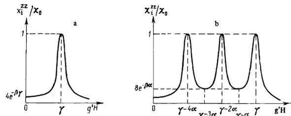
FIG. 3. Dependence of  $\chi$  on  $H$ : a)  $S' = 1/2, T \ll \gamma$ ; b)  $S' = 3/2, T \ll \alpha$ .
