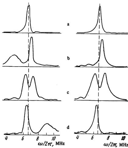
FIG. 5. Frequency spectra of oscillations of the field  $H_z$  (at the left) and the high-frequency current (at the right) without plasma a) and in plasma: b) for  $H < H_1$ , c) for  $H_0 = H$  and d) for  $H > H_2$ . The vertical dashed lines denote the frequency of the characteristic oscillations of the circuit without the plasma.
