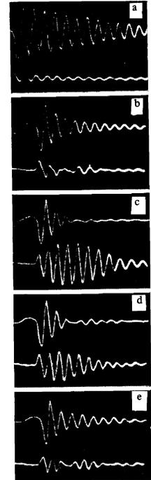
FIG. 4. Oscillograms of the high-frequency current in the coil (upper trace) and the field  $H_z$  on the axis: a) without plasma; b) for  $H < H_1$ ; c) for  $H = H_1$ ; d) for  $H = H_0$ ; e) for  $H > H_2$ .
