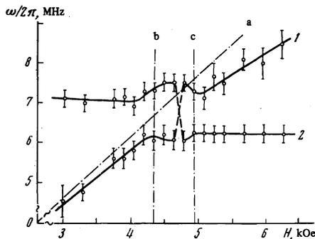
FIG. 6. Dependence of the frequency of oscillations excited in the plasma on the intensity of the constant magnetic field. The straight line a denotes  $\omega_H/2\pi$ , b, c—the locations of the absorption maxima.
