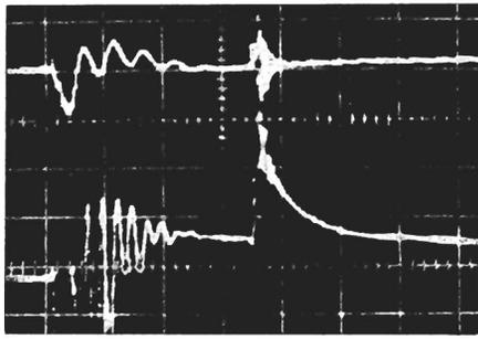
FIG. 2. Upper trace—simultaneous oscillograms of the direct discharge current and the high-frequency current; lower trace—diamagnetic signal; scale—5  $\mu$ sec/div.
