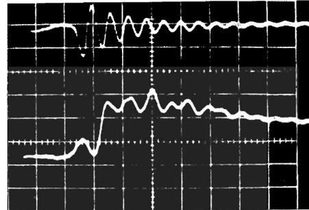
FIG. 11. The high-frequency current in the excitation coil (upper trace) and the diamagnetic signal: scale—0.25  $\mu\text{sec}/\text{div}$ .
