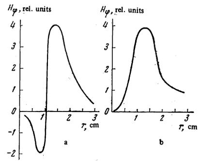
FIG. 7. Distribution of  $H_\phi(r)$  in plasma, obtained with the help of an 8-turn probe.
