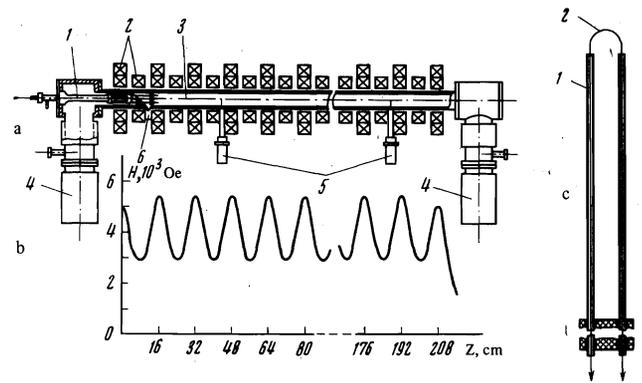
FIG. 2. a) Diagram of experimental setup: 1) ionizer; 2) magnetic-field coils; 3) vacuum volume; 4) magnetic-discharge pumps; 5) probes; 6) setup for the inlet of cesium vapor. b) Profile of magnetic field at the systems axis. c) Construction of incandescent probe: 1—quartz capillary; 2—tungsten filament.
