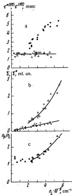
FIG. 6. Results of pulse measurements: a—dependence of plasma half-lives  $\tau_9^{(1/2)}$  (O) and  $\tau_9^{(1/2)}$  ( $\Delta$ ) on the concentration  $n_L$  at the last probe for the case of corrugated and homogeneous magnetic fields; b—plots of  $\Sigma(n_L)$  (O) and  $\Sigma^*(n_L)$  (+) obtained by graphic integration of the oscillograms; c—effect of corrugation of the magnetic field on the longitudinal density drop. (Reduction of the stationary sections of the oscillograms.)
