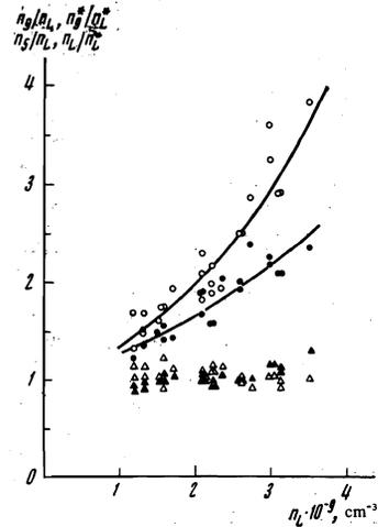
FIG. 3. Effect of corrugation of the magnetic field on the longitudinal density drop ( $n_L$  is the plasma concentration at the exit from the installation,  $n_5$  and  $n_9$  are the concentrations at distances of five and nine probkotrons from the end of the system, respectively):  $\circ$ — $n_9/n_L$ ,  $\bullet$ — $n_5/n_L$ ,  $\Delta$ — $n_L/n_L^*$ ,  $\blacktriangle$ — $n_9^*/n_L^*$ . The asterisks mark quantities corresponding to the homogeneous magnetic field.
