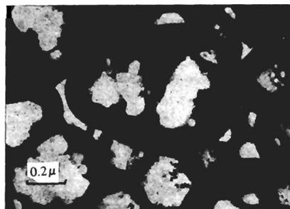
FIG. 4. Electron microgram of a polymer film formed by Ne<sup>+</sup> ions on a copper substrate ( $\times 50\,000$ ).
