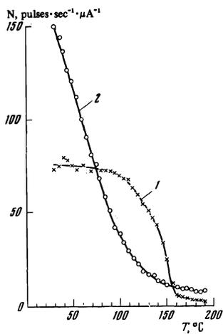
FIG. 5. Dependences of the intensity of the luminescence of neon atoms and molecules on the temperature of the polymer film: 1—atomic line Ne I  $\lambda = 5852\text{\AA}$ ; 2—molecular band of  $\text{Ne}_2$ ,  $\lambda = 5400\text{\AA}$ .
