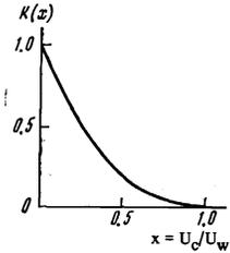
FIG. 4. VCN yield as a function of the ratio of the converter and neutron-guide wall potentials ( $U_c/U_w$ ).
