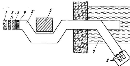
FIG. 5. VCN channel scheme for the IBR-30 pulsed reactor. 1—active zone of the reactor, 2—water moderator, 3—converter, 4—additional moderator, 5—copper neutron guide, 6, 7—shield and direct beam trap, 8—VCN deflectors.
