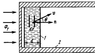
FIG. 1. Initial part of the neutron guide for very cold neutrons: 1—VCN converter exposed to the isotropic neutron flux, 2—vacuum neutron guide.
