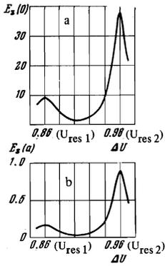
FIG. 10. Calculated dependence of field amplitude  $E_z$  vs the plasma density for  $V_{ph} \sim$  c: a—on the axis of the waveguide, b—at the boundary;  $U \equiv \omega_p^2/\omega^2$ ,  $U_{res} \equiv \omega_p^2/\omega M^2$ ,  $\Delta U = U - U_{res}$ .
