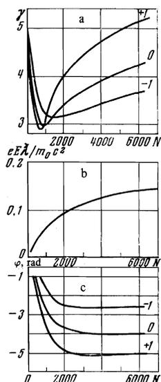
FIG. 11. Theoretical plots of the time variation of a) the energy loss, b) the field amplitude, c—the field phase; -1) beginning of bunch, 0) middle of bunch, +1) end of bunch.
