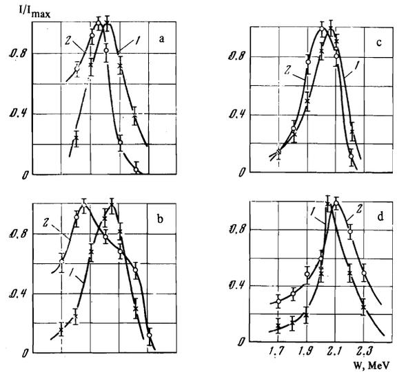
FIG. 5. Time variation of beam spectrum without (1) and with (2) plasma: a— $t = 0.3$  msec, b— $t = 0.5$  msec, c— $t = 1.0$  msec, d— $t = 1.6$  msec.
