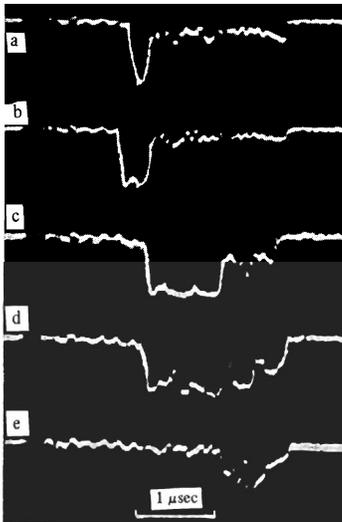
FIG. 4. Current oscillograms of an electron beam that has traversed the plasma, for different sections of the spectrum: a— $W = 1.7$  MeV, b— $W = 1.8$  MeV, c— $W = 2.0$  MeV, d— $W = 2.2$  MeV, e— $W = 2.3$  MeV.
