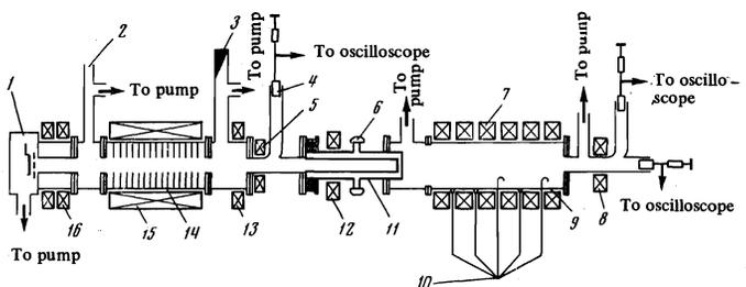
FIG. 1. Block diagram of the apparatus: 1—electron gun, 2—vacuum waveguide, 3—microwave load, 4—Faraday cylinder, 5, 8, 12, 13, 16—beam correction and focusing systems, 6—electrodynamical valve, 7, 15—solenoids, 9—interaction chamber, 10—microwave diagnostics elements, 11—plasma gun, 14—iris-loaded waveguide.
