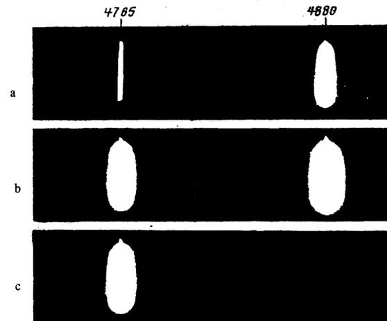
FIG. 6. Dependence of the intensity of the generation lines on the argon pressure  $P_0$  visible region; chamber of diameter 10 cm): a)  $P_0 = 6 \times 10^{-4} \text{ Torr}$ ; b)  $P_0 = 7 \times 10^{-4} \text{ Torr}$ ; c)  $P_0 = 8 \times 10^{-4} \text{ Torr}$ .
