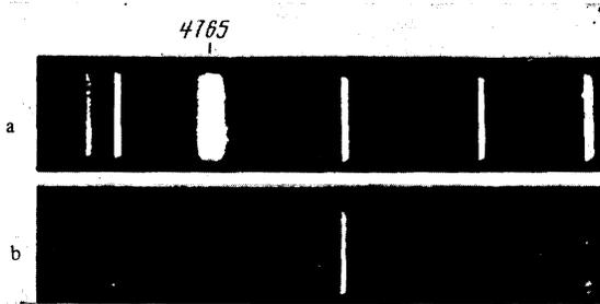
FIG. 5. Section of radiation spectrum (visible region; chamber of diameter 10 cm): a) electron beam directed towards the region B; b) electron beam directed towards the electrode 4 (Fig. 1). The exposure (number of discharges) was the same in both cases.
