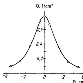
FIG. 2. Electron beam energy density distribution over the cross section of the discharge chamber (diameter 10 cm).
