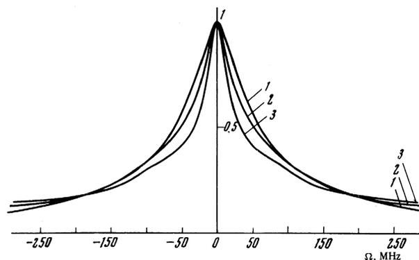
FIG. 2. Spectrograms of the absorption coefficient: 1—identical linear or circular polarizations, 2—perpendicular linear polarization, 3—opposing circular polarizations.
