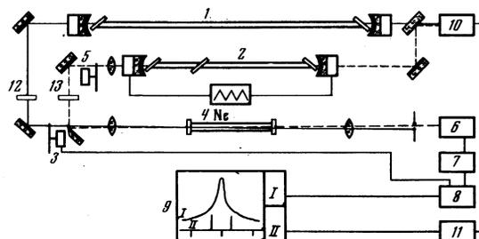
FIG. 1. Diagram of experimental setup: 1, 2—He-Ne laser; 3, 5—modulator; 4—gas-discharge cell; 6, 10—photomultiplier; 7, 8—selective amplifier with detector; 9—automatic recorder; 11—radio receivers; 12, 13—phase plates.
