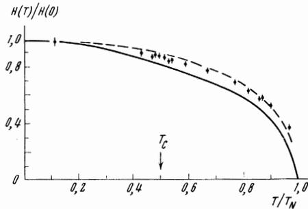
FIG. 3. Temperature dependence of the magnetic field for Dy nuclei in metallic Dy. The solid curve is the Brillouin curve for  $J = 15/2$ . The dashed curve is calculated from formula (4).
