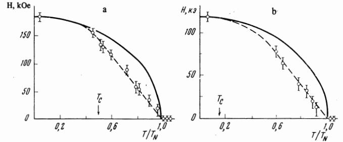
FIG. 2. Temperature dependence of the magnetic field at the nuclei of Sn impurity atoms in metallic Dy (a) and in metallic Ho (b). The solid curves are Brillouin curves for  $J = 15/2$  and  $J = 8$  respectively.
