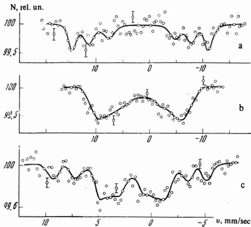
FIG. 1. Spectra of the resonance absorption of  $\gamma$ -quanta by nuclei of  $\text{Sn}^{119}$  impurity atoms in Dy (a), Ho (b) and Tm (c), measured at temperature  $7^\circ\text{K}$ . The speed of the source of  $\gamma$ -quanta is plotted along the abscissa, and the intensity of the flux of quanta in relative units along the ordinate.
