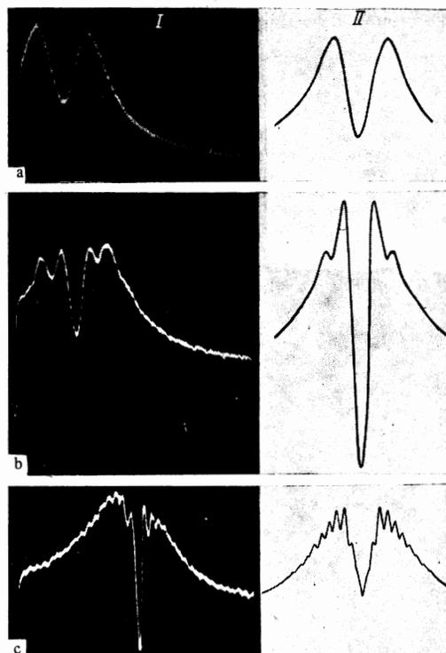
FIG. 2. Oscillograms of the PTS (left) and calculated PTS shapes (right) for the following microwave pulse durations: a)  $\tau = 4 \times 10^{-7}$  sec, b)  $\tau = 8 \times 10^{-7}$  sec, c)  $\tau = 2.5 \times 10^{-6}$  sec.
