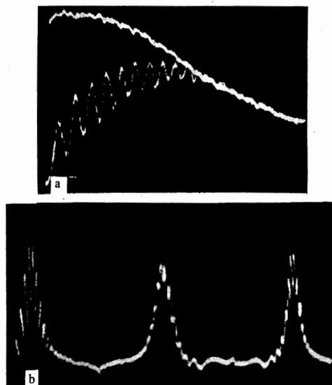
FIG. 1. a) Oscillogram of a portion of the equilibrium EPR line-shape of nitrogen in SiC (upper) and the PTS pattern (lower) arising in it after the action of a microwave pulse. b) Oscillogram illustrating the "filling in" of the PTS in the course of a few cycles of the magnetic modulation (50 Hz, nitrogen concentration  $5 \times 10^{17}$  cm<sup>-3</sup>).
