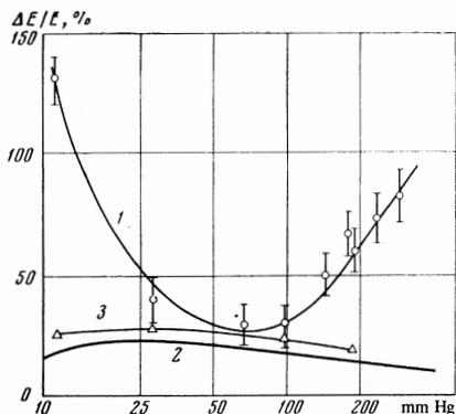
FIG. 1. Pressure dependence of the relative increase of the stimulated-emission energy yield: O—CF<sub>3</sub>I, Δ—C<sub>3</sub>F<sub>7</sub>I.
