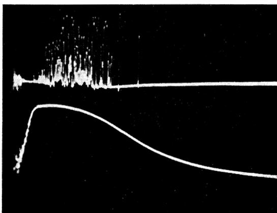
FIG. 3. Oscillograms of generation pulse and pump pulse with selective additional illumination.
