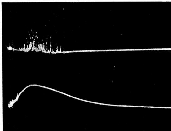
FIG. 2. Oscillograms of generation pulse and of pump pulse without selected additional illumination.
