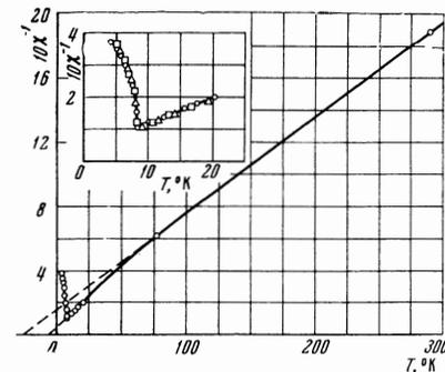
FIG. 1. Temperature dependence of the magnetic susceptibility of single-crystal NdS:  $\circ$ —H || [100],  $\triangle$ —H || [010],  $\square$ —H || [111].
