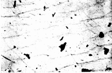
FIG. 2. Domain structure obtained by evaporating iron particles on the (100) plane of single-crystal NdS. Magnification  $10^4 \times$ .
