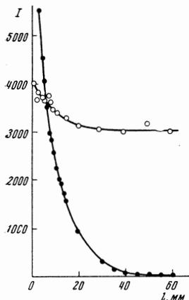
FIG. 2. Graphs of  $I(l)$ : ●—the  $\lambda 3914$  band of the first negative system of  $N_2^+$  ions; ○—the  $\lambda 3994$  band of the second positive system of  $N_2$  molecules (with relative units for  $I$ ).
