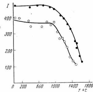
FIG. 3. Intensity (in relative units) versus temperature: ●—the  $\lambda 3914$  band of the first negative system of  $N_2^+$ ; ○—the  $\lambda 4272$  band of the system of comet tail bands of  $CO^+$ .
