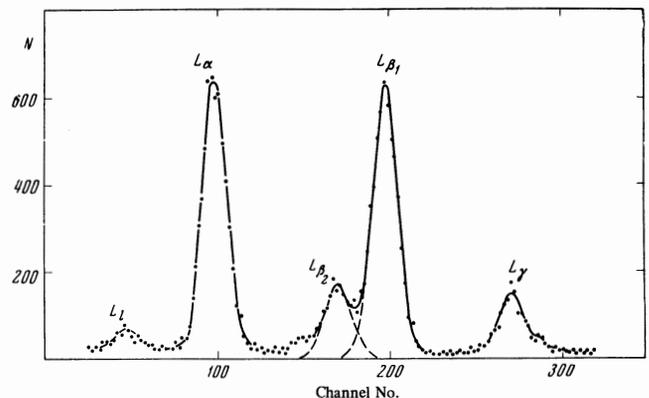
Spectrum of L series of characteristic radiation of <sup>248</sup>Cm in the  $\alpha$  decay of <sup>252</sup>Cf. The dashed lines show the results of the graphic separation of the lines L<sub>3</sub> and L<sub>4</sub>.
