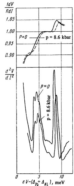
FIG. 1. Sample plots of the quantities  $R^{-1}dV/dI$  and  $d^2V/dI^2$  as functions of  $V$  for lead at  $P = 0$  and  $P = 8.6$  kbar.
