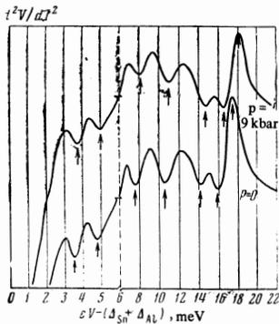
FIG. 2. Sample plots of the d<sup>2</sup>V/dI<sup>2</sup> characteristics for tin in arbitrary units at P = 0 and P = 9 kbar. The scale changes at 6 meV.
