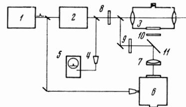
FIG. 1. Experimental setup: 1) ruby laser, 2) optical amplifier, 3) chamber with focusing lens, 4) coaxial photocell, 5) fast oscillograph, 6) image converter, 7) objective, 8)-9) optical filters, 11) glass plate.
