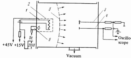
FIG. 5. Experimental setup: 1—incandescent cathode, 2—anode, 3—emission probe, 4—Langmuir probe, 5—profile of gas cloud, 6—pulsed valve.
