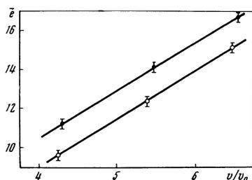
FIG. 1. Velocity dependence of mean charge for  $\text{Kr}^{84}$  ions: ●—in air (0.35 Torr), ○—in He (2.7 Torr).
