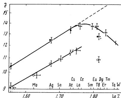
FIG. 2. Dependence of mean charge on  $Z$  ( $v/v_0 = 4$ ): ●—in air (0.35 Torr), ○—in He (2.7 Torr).
