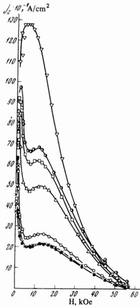
FIG. 7. Anisotropy of critical current in a recrystallized wire sample made of the alloy Ti-22 at.% Nb and subjected to the following aging for one hour at  $t = 380^\circ\text{C}$ , diameter 0.114 mm,  $\bullet$ — $\alpha = 90^\circ$ ,  $\times$ — $\alpha = 73^\circ$ ,  $\circ$ — $\alpha = 53^\circ$ ,  $\Delta$ — $\alpha = 22.5^\circ$ ,  $\square$ — $\alpha = 10.5^\circ$ ,  $\bullet$ — $\alpha = 6^\circ$ ,  $\nabla$ — $\alpha = 0^\circ$ .
