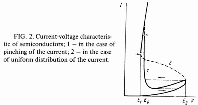
FIG. 2. Current-voltage characteristic of semiconductors; 1 — in the case of pinching of the current; 2 — in the case of uniform distribution of the current.
