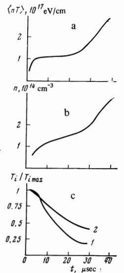
FIG. 4. Quantities calculated for the initial stage of the discharge: a – running energy density in the discharge  $\langle nT \rangle$ , b – plasma concentration  $n(t)$ , c –  $T_1(t)/T_{1\text{max}}$  (curve 1) and  $T_2(t)/T_{2\text{max}}$  (curve 2). The time dependence of  $T_{1,2}(t)/T_{1,2\text{max}}$  is calculated from the oscillograms of the flux of atoms with energies 100 eV and 4.5 keV, respectively.
