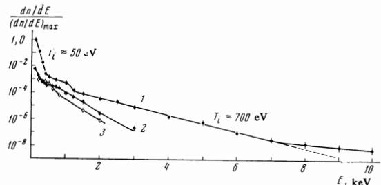
FIG. 3. Energy distribution function of hydrogen ions. 1 –  $t = 0$ , 2 –  $t = 50$   $\mu$ sec, 3 –  $t = 100$   $\mu$ sec. The curves are normalized to the value of  $(dn/dE)_{max}$  corresponding to  $dn/dE$  at  $t = 0$  and  $E = 100$  eV.
