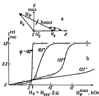
FIG. 2. The geometry of experiment (a) and its result (b)—the dependence of the relative oscillation amplitude on the pulsed field and its orientation relative to the constant field.
