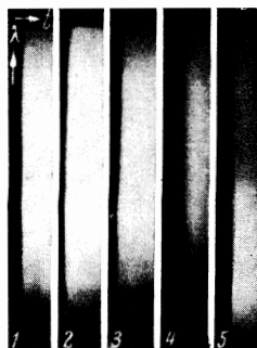
FIG. 3. Spectrophotochronograms of the radiation of shock waves, \lambda = 230-430 nm: 1 - Xe, 2 - Kr, 3 - Ar, 4 - Ne, 5 - Ar, \lambda = 460-660 nm.
