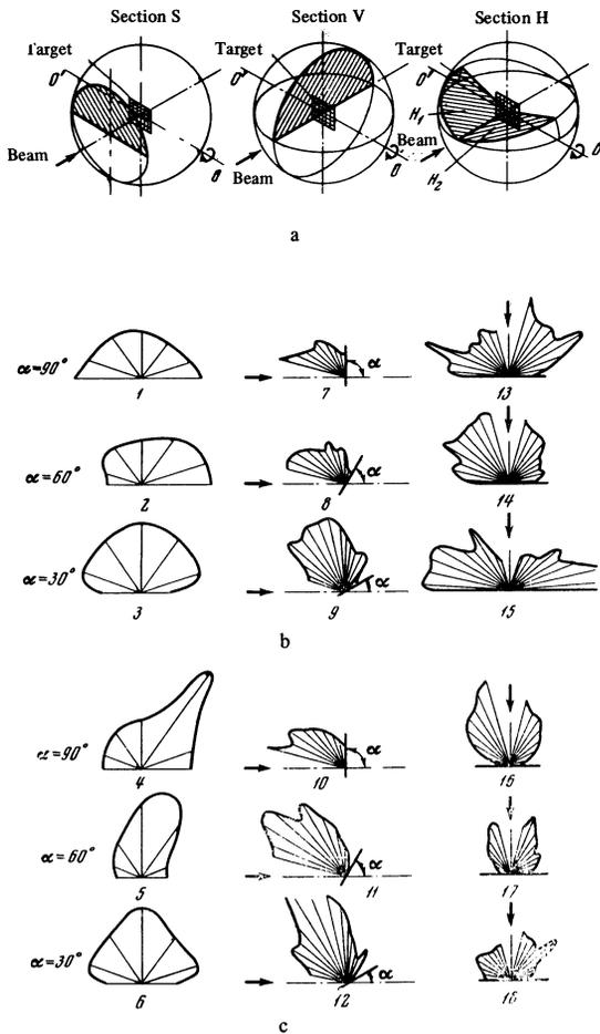
Geometry of the experiment (A) and experimental results in free-running (B) and Q-switched (C) operation. Diagrams of Section (B) show activity distribution along the line of intersection of the spherical chamber with plane S located 40 mm away from the target; diagrams V refer to intersection with plane V; and diagrams H refer to intersection with planes H<sub>1</sub> and H<sub>2</sub> inclined at 18° to the horizontal plane.
