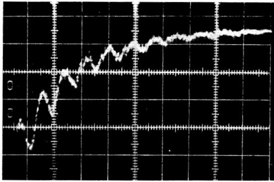
FIG. 2. Oscillogram of the oscillations of the intensity of the afterglow in helium plasma upon cooling of the discharge tube to  $4^\circ\text{K}$  ( $4650 \text{ \AA}$  band).  $N = 3 \times 10^{17} \text{ cm}^{-3}$ , radius of retort,  $R = 2 \text{ cm}$ ,  $\tau = 5 \text{ \mu sec}$  (along ordinate: intensity in arbitrary units, scale along the time axis, one unit corresponds to  $200 \text{ \mu sec}$ ; O – start of sweep).
