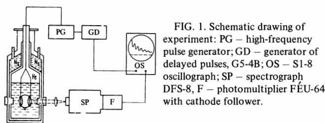
FIG. 1. Schematic drawing of experiment: PG — high-frequency pulse generator; GD — generator of delayed pulses, G5-4B; OS — S1-8 oscillograph; SP — spectrograph DFS-8, F — photomultiplier FÉU-64 with cathode follower.
