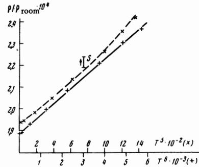
FIG. 6. Electric resistivity  $\rho$  as the function of  $T^5$  (X) and  $T^6$  (+). The  $\rho(T^5)$  curve is shifted upward along the ordinate axis by a distance S.
