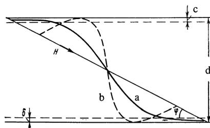
FIG. 2. Curve a—boundary orbit separating the effective orbits from the ineffective ones<sup>[14]</sup>, b—orbit with two effective points per period.
