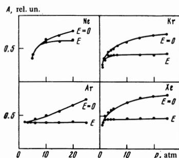
FIG. 9. Dependence of the scintillation amplitude  $A$  of various noble gases under the influence of  $\alpha$ -particles on the gas pressure  $p$ . The curves were plotted without a field ( $E = 0$ ) and in the presence of a field ( $E$ ) ensuring the maximum decrease of the scintillation amplitude.
