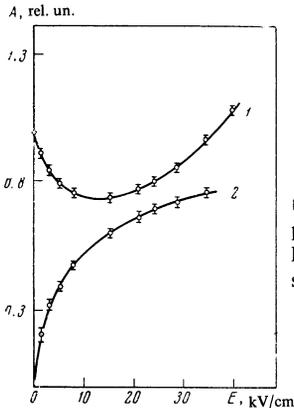
FIG. 1. Amplitude A of scintillations (curve 1) and of the ionization pulse (curve 2) vs. the electric field E. Ionization by  $\alpha$ -particles, xenon density  $0.66 \text{ g/cm}^3$ .
