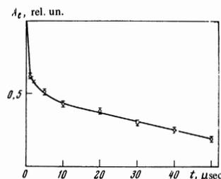
FIG. 6. Decrease of electroluminescence amplitude  $A_e$  with time. Xenon ( $\rho = 0.3 \text{ g/cm}^3$ ) ionized by an x-ray pulse.
