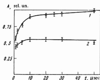
FIG. 5. Growth of the amplitude  $A$  of the scintillation pulse with time. Xenon ( $\rho = 0.3 \text{ g/cm}^3$ ) ionized with an x-ray pulse. Curve 1—electric field off, curve 2—electric field of 3 kV/cm turned on.
