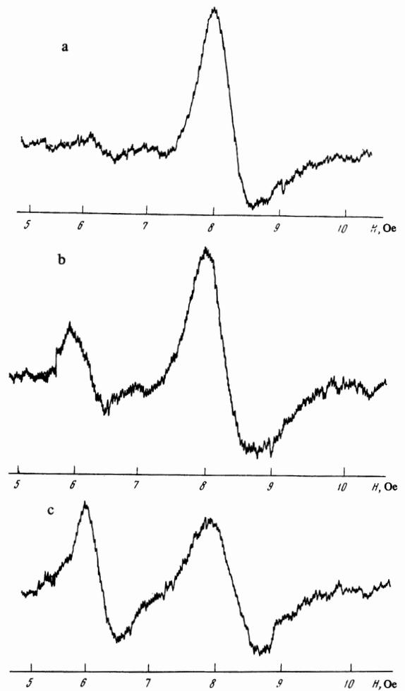
FIG. 2. Example of the dependence of the ratio of the hyperfine components of the signal on the discharge current. a—40 mA, b—50 mA, c—60 mA.
