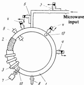
FIG. 1. Diagram of the L-1 stellarator and location of the various elements: 1 - stellarator vacuum chamber, 2 - helical winding, 3 - longitudinal field coil, 4 - pickup unit for measuring the level of the microwave field, 5, 6 - directional couplers, 7 - plasma injector, 8 - Langmuir probe, 9 - microwave diagnostics, 10 - pickup unit for pulsed measurements of the pressure inside the vacuum chamber.
