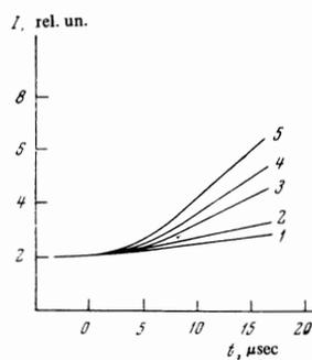
FIG. 5. Curve showing the time variation in ion saturation current to the probe during the heating pulse for various microwave power levels: 1 - 250 W, 2 - 400 W, 3 - 600W, 4 - 1kW, 5 - 1.8 kW.
