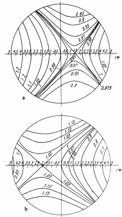
FIG. 2. Magnetic isobars for the L-1 stellarator for  $\epsilon = 0.33$ . The major axis of the elliptic magnetic surface is oriented as follows: a) vertical, b) horizontal.
