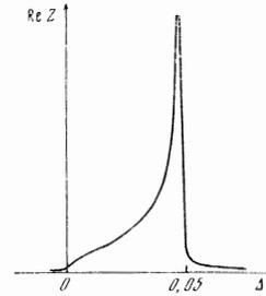
FIG. 4. Behavior of the real part of the surface impedance in the vicinity of the cyclotron resonance for values  $\xi = 1$ ;  $\gamma = 0.001$ , and  $Z_0 = 4\pi\omega\delta_0 c^2$ .
