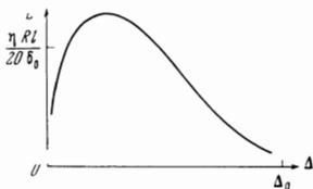
FIG. 2. Dependence of the damping length of the long-wave branch of the cyclotron wave on the value of  $\Delta$ .
