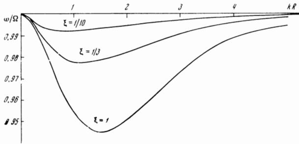
FIG. 1. Spectral curves of the ordinary cyclotron wave for values of  $\xi$  equal to 1/10, 1/3, and  $l \rightarrow \infty$ .
