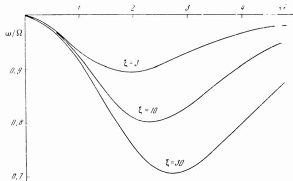
FIG. 3. Spectral curves of the cyclotron wave for  $\xi$  equal to 3, 10, and 30 as  $l \rightarrow \infty$ .
