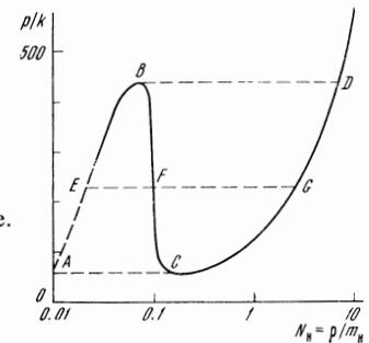
FIG. 1. The dependence of the stationary pressure on the density. The region BC is unstable.
