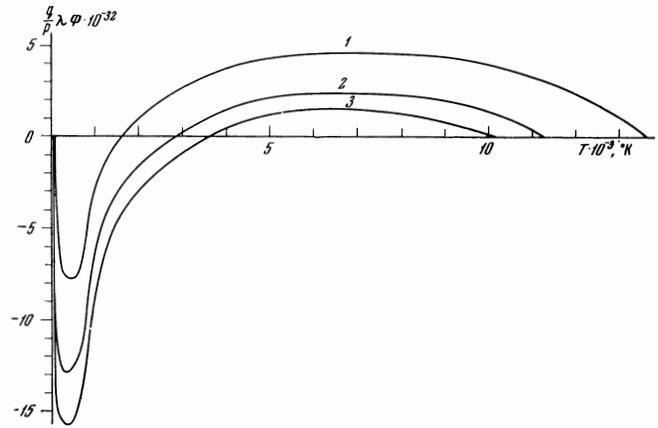
FIG. 3. The curves representing  $q\lambda\Phi/p$  as a function of  $T$  for various values of the parameter  $p/q$ : 1 -  $7 \times 10^{11}$ , 2 -  $11 \times 10^{11}$ , 3 -  $14 \times 10^{11}$  cgs esu.
