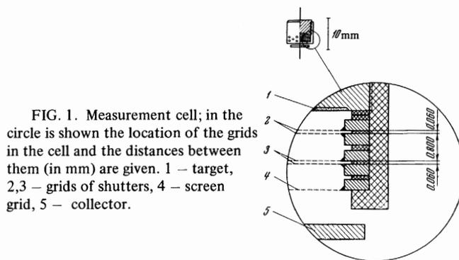
FIG. 1. Measurement cell; in the circle is shown the location of the grids in the cell and the distances between them (in mm) are given. 1 - target, 2,3 - grids of shutters, 4 - screen grid, 5 - collector.
