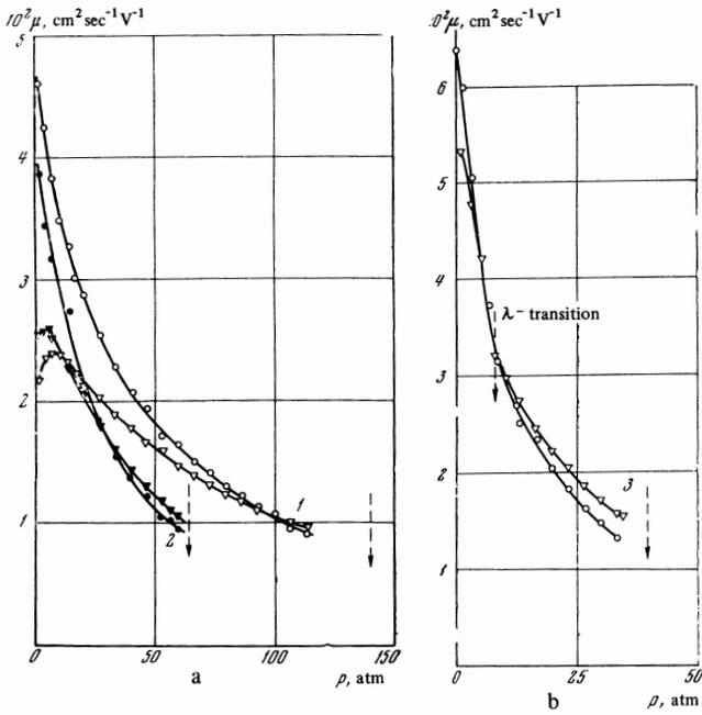
FIG. 2. Pressure dependence of the mobility of the charges in liquid helium. The circles correspond to positive charges, the triangles to negative ones. Curves 1 and 2 were obtained for temperatures of 4.2 and 2.63°K, respectively, curves 3 were obtained for a temperature of 2.07°K. The arrows indicate the solidification pressure for a given temperature.
