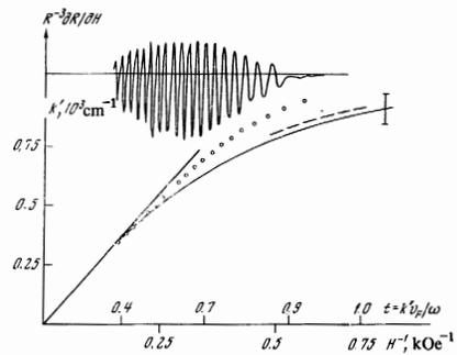
FIG. 2. Spectrum of the wave for strong spatial dispersion. Points—data of experiment for 9.62 GHz,  $\mathbf{k} \parallel \mathbf{C}_2$ ,  $\mathbf{H} \perp \mathbf{C}_3 \parallel \mathbf{J}$ ,  $\chi = 4^\circ 40'$ . Continuous curve—calculation for  $\omega/\Omega \ll 1$ , dashed curve—with account of the correction for time dispersion. Straight line—asymptote as  $H^{-1} \rightarrow 0$ . The vertical bar indicates the accuracy of the calculation.
