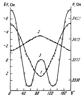
FIG. 1. Angular dependencies: 1 — of the shift of the resonance field  $\delta H(\theta, k_1)$  for single-crystal ferrites  $\text{Li}_{0.5}\text{Fe}_{2.07}\text{Ga}_{0.43}\text{O}_4$  (at  $\sigma = 60 \times 10^6$  dyne/cm<sup>2</sup>); 2 — of the shift of the resonance field  $\delta H(\theta, k_1)$  for yttrium ferrites (at  $\sigma = 87 \times 10^6$  dyne/cm<sup>2</sup>); 3 — of the resonant field  $H(\theta)$  for yttrium ferrites.
