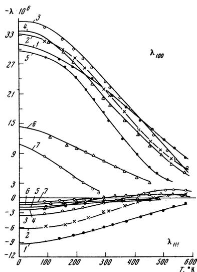
FIG. 2. Temperature dependence of the magnetostriction constants  $\lambda_{100}$  and  $\lambda_{111}$  of single-crystal ferrites  $\text{Li}_{0.5}\text{Fe}_{2.5-x}\text{Ga}_x\text{O}_4$ : 1 -  $x = 0$ ; 2 -  $x = 0.06$ ; 3 -  $x = 0.16$ ; 4 -  $x = 0.43$ ; 5 -  $x = 0.65$ ; 6 -  $x = 0.9$ ; 7 -  $x = 1.18$
