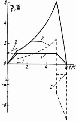
FIG. 6. Plots of the reduced phases  $\tilde{\varphi} = K\varphi_{1a}(K = -\nu_+/\sigma_{12} I_{20})$  (solid curves) and of the reduced deviation of the carrier frequency  $\tilde{\Omega} = K \partial\varphi_{1a}/\partial t$  (dashed) at the different values of  $\alpha$ : 1 -  $\alpha = 0$ , 2 -  $\alpha = 0.2$   $\nu_+/\tau(\nu_+ L = 5\tau)$ .
