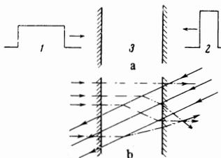
FIG. 5. a - interaction of pulses 1 and 2 in a cubic medium; b - spatial analog of Fig. a - interaction of bounded beams of weak wave of frequency  $\omega_1$  are shown dashed; rays of intense wave of frequency  $\omega_2$  - solid.
