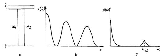
FIG. 1. a - Model level scheme, b - time variation of the spontaneous emission in the case of interference between the states 1 and 2, c - beat-power spectrum.
