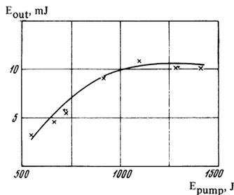
FIG. 4. Output emission energy as a function of pump energy in giant pulse mode.
