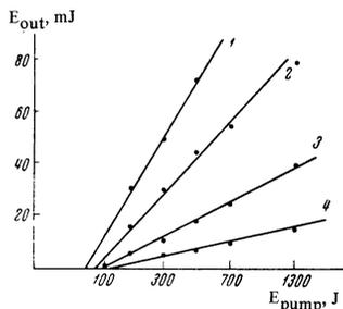
FIG. 3. Output emission energy as a function of pump energy in free-running mode: 1 – no shutter elements in resonator; 2 – a single Glan prism in resonator; 3 – two Glan prisms with parallel oscillation planes; 4 –  $\text{LiNbO}_3$  crystal in crossed Glan prisms.
