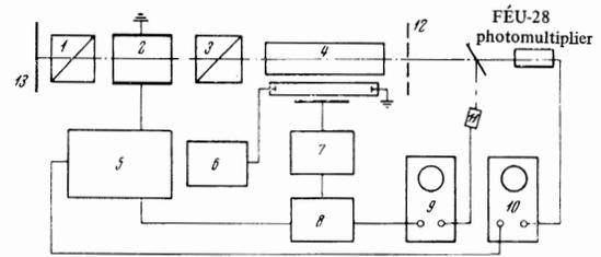
FIG. 1. Diagram of experimental setup: 1, 3 – Glan prisms; 2 –  $\text{LiNbO}_3$  crystal; 4 –  $\text{CaF}_2:\text{Dy}^{2+}$  crystal; 5 – high-voltage pulse generator; 6 – charging circuit; 7 – starting circuit; 8 – G5-15 generator with delay line; 9 – SI-16 oscilloscope; 10 – SI-11 oscilloscope; 11 – PbS photoresistor; 12 – quartz substrates; 13 – mirror with  $R = 100\%$
