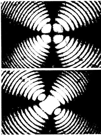
FIG. 2. Conoscopic pictures of the  $\text{LiNbO}_3$  crystal in crossed polaroids: a – corresponds to minimum transmission with zero field on crystal; b – corresponds to the first transmission maximum at  $V = V_{\lambda/2}$ .
