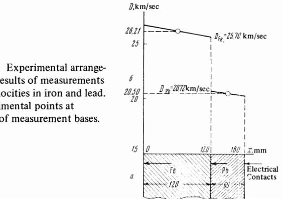
FIG. 1. Experimental arrangement and results of measurements of wave velocities in iron and lead. O — experimental points at midpoints of measurement bases.
