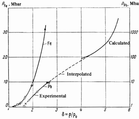
FIG. 3. P -  $\delta$  diagrams of the standard adiabat of lead and of the experimental adiabat of iron.  $\square$  - unpublished results of the present authors. The rest of the notation is the same as in Fig. 2.
