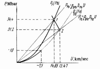
FIG. 4. Schematic diagram used to determine the shock-compression parameters of iron
