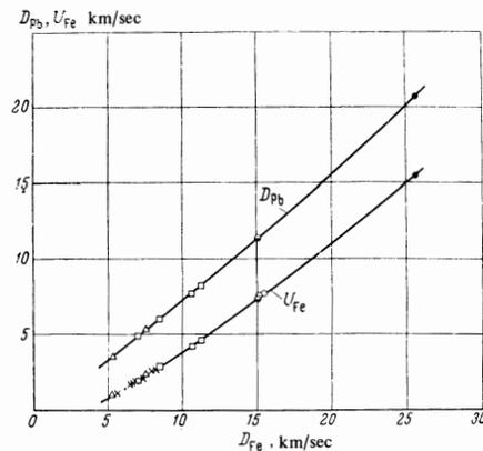
FIG. 2. Experimentally determined dependences  $D_{Fe} = f(D_{Pb})$  (upper curve) and  $D_{Fe} = f(U_{Fe})$  (lower curve). ● — results of present investigation; Δ — [1]; □ — [2]; ● — [4]; ○ — [5]; × — [7].
