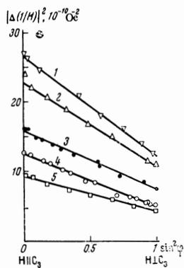
FIG. 6. Dependence of period of oscillation (in the scale of the reciprocal field) on  $\sin^2 \varphi$ . The straight lines correspond to Eq. (2),  $T = 1.5^\circ \text{K}$ .
