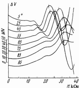
FIG. 3. Dependence of the transverse magnetoresistance of tellurium on the field for different angles between  $H$  and  $C_3$ , without commutation of the field; the sample No. 5,  $T = 1.5^\circ K$ . The value of the measured signal  $\Delta V$ , which is proportional to  $\Delta\rho/\Delta\rho_0$  is plotted along the ordinate. The position of the first maximum of the oscillating component of  $\rho(H)$  is indicated by the vertical lines.
