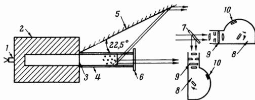
FIG. 2. Experimental arrangement (not drawn entirely to scale; the charge and mirror are arbitrarily rotated  $90^\circ$  about the tube axis). 1—electrodetonator, 2—charge with cumulative channel, 3—cellophane diaphragm, 4—glass tube (1.5 cm diameter) containing experimental gas, 5—mirror, 6—quartz end-window, 7—half-silvered mirror, 8—camera, 9—color filter, 10—step attenuator.
