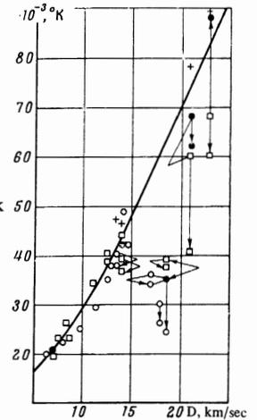
FIG. 5. Brightness temperature of shock front in argon (with the same symbols as in Fig. 4.)
