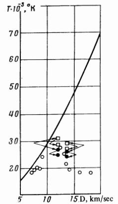
FIG. 7. Brightness temperature of shock front in a mixture of argon and air. The air admixture was 5% for the measurements in the ultraviolet and yellow regions. The curve represents the calculated post-shock temperature for argon. The brightness temperature for blue light was not measured at 45°. Otherwise the symbols are as in Fig. 4.
