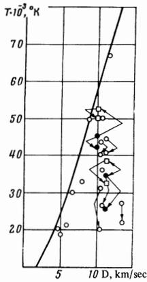
FIG. 6. Brightness temperature of shock front in xenon (with the same symbols as in Fig. 4).
