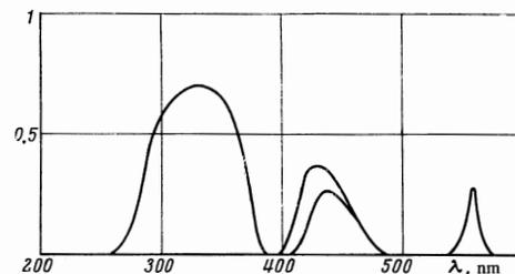
FIG. 1. Transmission curves of the color filters.
