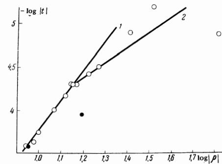
FIG. 3. Coexistence curve of helium in the immediate vicinity of the critical point. Line 1 corresponds to  $(-t) \sim |\rho|^3$  and line 2 to  $(-t) \sim \rho^2$ . Experimental points: [22] ○—gas, ●—liquid.
