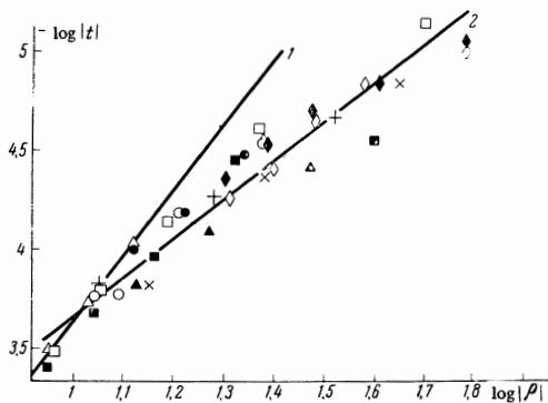
FIG. 1. Coexistence curve for  $\text{C}_2\text{H}_4$ ,  $\text{Xe}$ , and  $\text{SF}_6$  in the immediate vicinity of the critical point. Line 1 corresponds to  $(-t) \sim |\rho|^3$ , and line 2 to  $(-t) \sim \rho^2$ ; experimental points:  $\text{C}_2\text{H}_4^{[12]}$ , ●—gas, ○—liquid at  $H_m = 15 \text{ cm}$ , ×—gas, +—liquid at  $H_m = 6 \text{ cm}$ ;  $\text{Xe}^{[19]}$ , ■—gas, □—liquid;  $\text{Xe}^{[12]}$ , ▲—gas, △—liquid;  $\text{SF}_6^{[23]}$ , ♦—gas, ◇—liquid.
