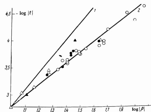
FIG. 2. Coexistence curve of  $\text{Cl}_2$  and  $\text{SF}_6$  in the immediate vicinity of the critical point. Line 1 corresponds to  $(-t) \sim |\rho|^3$  and line 2 to  $(-t) \sim \rho^2$ ; experimental points:  $\text{Cl}_2^{[21]}$ , ●—gas, ○—liquid;  $\text{SF}_6^{[20]}$ , ▲—gas, △—liquid.
